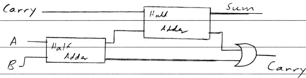
If two half adders are connected like above, with one the sum of the first half-adder feeding into the input of the second and the carry of both feeding into an OR gate, a full adder would have been created.
