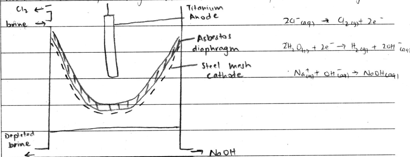
However, the  $\overset{\text{NaOH}}{\text{brine}}$  produced was contaminated with chlorine and the asbestos diaphragm was found to be harmful to humans. Thus further developments and ~~advancements~~ advancements in technology led to the membrane cell.
