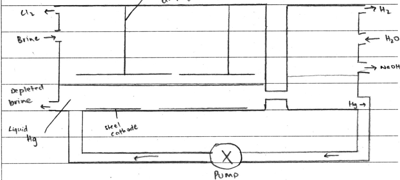
However, technical and environmental issues arose. The mercury that was theoretically supposed to be recycled was found to contaminate the NaOH produced, leading to environmental concerns as mercury is a heavy metal that accumulates in the body and causes
