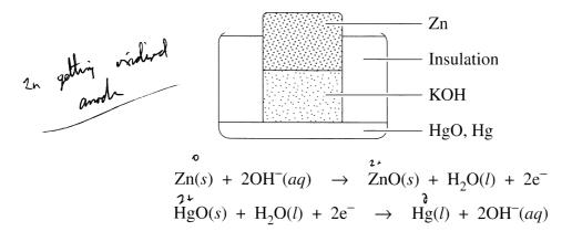
Identify the anode, cathode and electrolyte for this cell.
