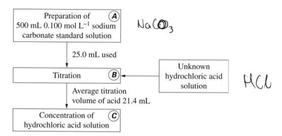
Describe steps **A**, **B** and **C** including correct techniques, equipment and appropriate calculations. Determine the concentration of the hydrochloric acid.
