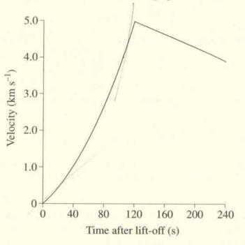
(a) Using either words or calculations, compare the acceleration of the rocket at t = 20 s with its acceleration at t = 100 s.
