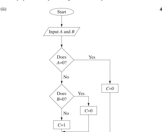
The flowchart above describes the logic of an AND gate where the values of *A* and *B* are binary digits.
