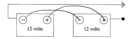
(e) In the diagram below, draw lines to show how to connect the terminals to maintain battery output voltage at 12 volts.
